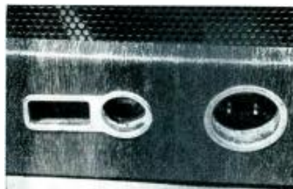
Above: the connection outlets are on the back of the recorder. Right: the pins which will shut off the recorder at the end of the tape if a loop has been formed around the hub of the reel.
