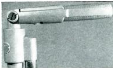
Above: The bi-directional pattern of the pickup plus the tilting feature will reduce unwanted noise and allow a PA system to be run about 6 db higher than usual when the "dead" sides of the mike are properly oriented in relation to the sound source. Right: showing the cable connection and impedance switch cover.
