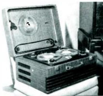
The line and microphone cords are wrapped on cleats in the lid and extra reels of tape are stored on the spring pins.
